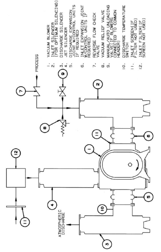
Figure 1 - Schematic Diagram
