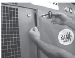
(2) Push and turn the key 1/4 turn clockwise, pull the door open.
