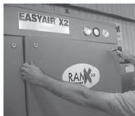
(4) Hold the door open with left hand, insert key in the right hole, push and turn the key 1/4 turn counter clockwise, pull the door open.
