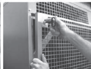
(6) For removal of the left door panel, use the procedure per (2 & 3) above to unlock the left latch, and (4 & 5) to unlock the right latch.
