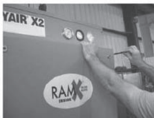
(5) Hold the door, push and turn the key 1/4 turn clockwise and remove the key. Lift up and remove the right side door panel.
